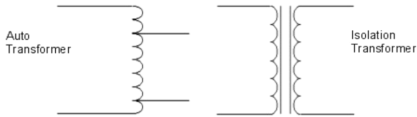
Figure 3.13 Typical connections in autotransformer vis-à-vis isolation transformer
